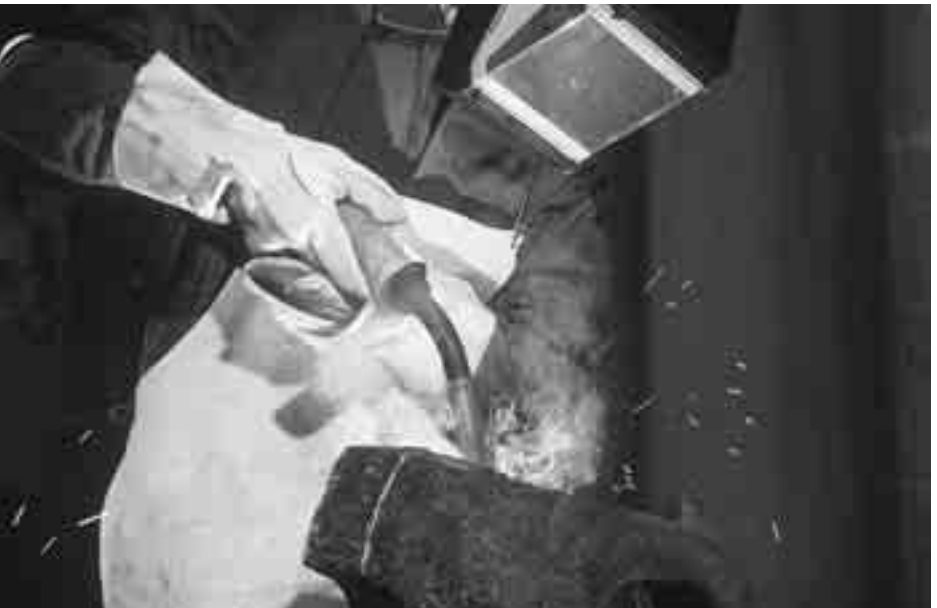
Hammerbrecher: OK Tubrodur 15.65
